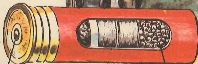
Cutaway view of standard load shotgun shell
